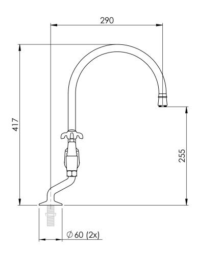
Holes to be drilled: 35 mm Maximum deck thickness: 35 mm
