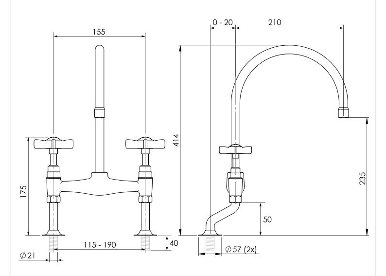
Hole to be drilled: 35 mm Maximum deck thickness: 20mm
