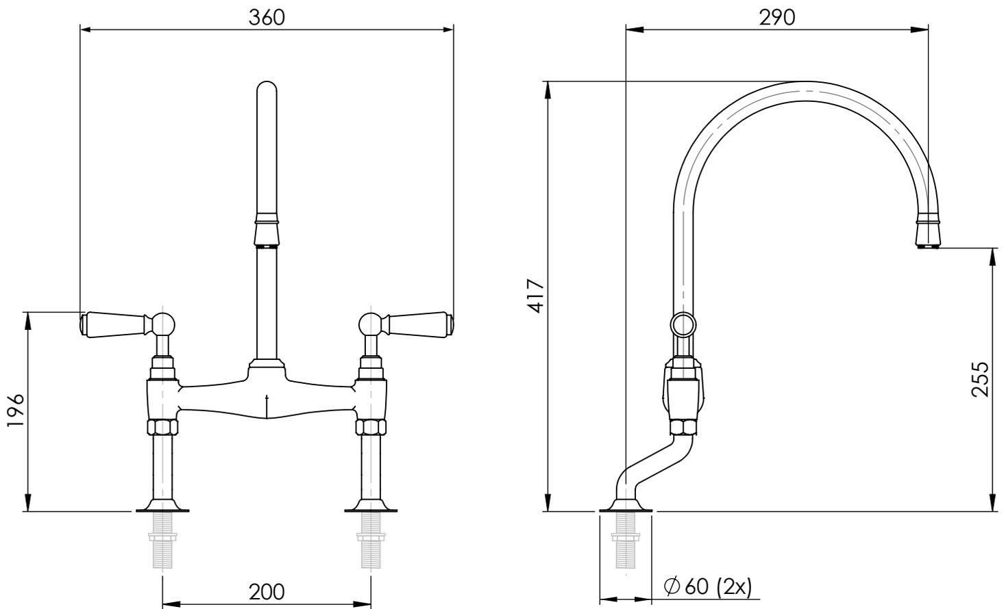
Holes to be drilled: 35 mm
