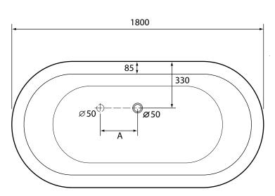
A: Floor connection evacuation tube at 150 - 600mm offset from crepine. Can be placed at either side of the crepine.
