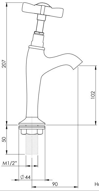
Holes to be drilled: 30 mm
