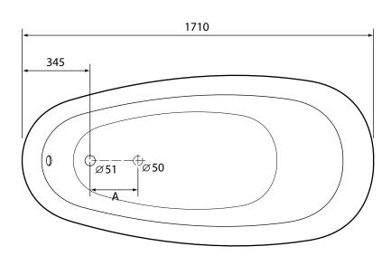
A: Floor connection evacuation tube at 150 - 600mm offset from crepine. Diameter evacuation tube in floor 50mm.
