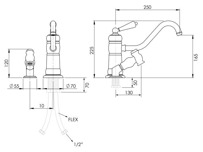
Sprayset hose: 1,5m Holes to drill: 35mm
