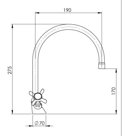
HOLES TO DRILL: 35MM MAXIMUM DECK THICKNESS: 45MM
